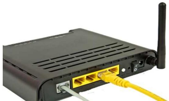
Fig: 4.18 DSL Modem
