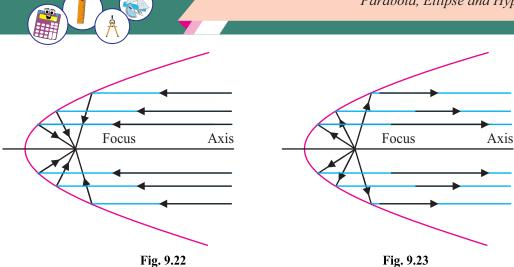
Conversely, if a light source is located at the focus of a parabolic reflector, then the reflected rays will form a beam of parallel rays parallel to the axis of parabola as shown in the figure 9.23. The parabolic reflectors in automobile headlights and flash light use this rule. The optical principles which have been discussed above are also valid for radar signals, sound waves, radio waves etc.
