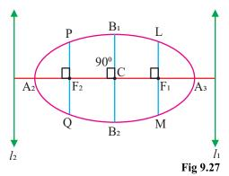
to the major axis is called minor axis. In the figure point C,  $\overline{A_1A_2}$  and  $\overline{B_1B_2}$  are the centre, major axis and minor axis of the ellipse respectively. The end points of major axis and minor axis are called vertices and covertices respectively.
