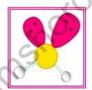
corners occupied by bond pairs. Since the lone pair repulsion is greater than bond pair repulsion, the two bond pairs deviate from the lone pair and come near to each other at 104.5°. This makes a distortion in the tetrahedral geometry and develops an angular shape.
